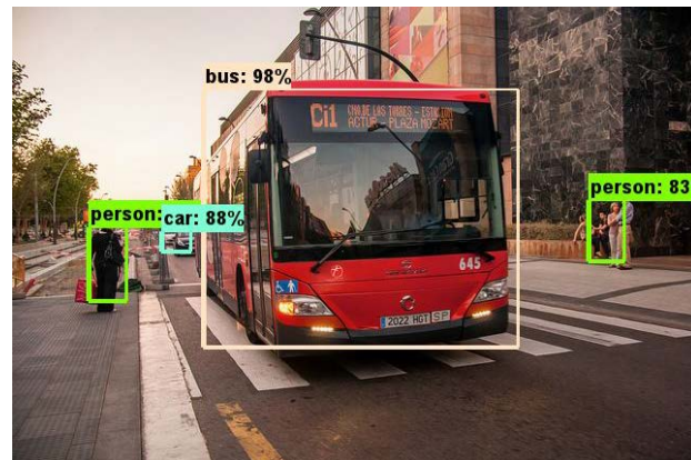
Abbildung 6: Example objection detection results using MobileNet SSD [b]
